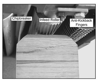
Figure 23. Feed roller height inspection.
